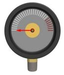
The Tensioner will have retracted upwards since the bolt will have elongated. The tool will need reengaging onto the flange.
