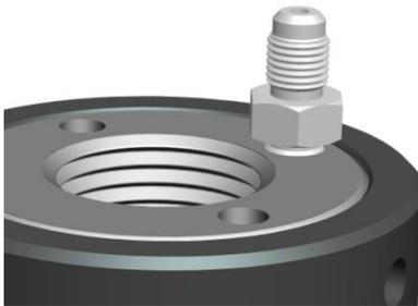
Screw the adaptor into the hydraulic Cylinder. The adaptor is identical at each end so it does not matter which end is inserted into the Cylinder.
