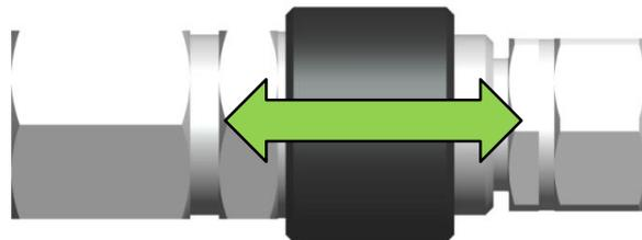
Coupling and nipple pushed together with the shroud retracted.
