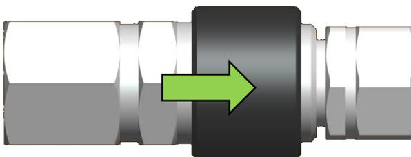
Shroud released, coupling and nipple are now locked together and safe to use.
