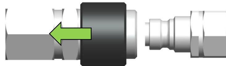
Coupling and nipple with the shroud retracted.
