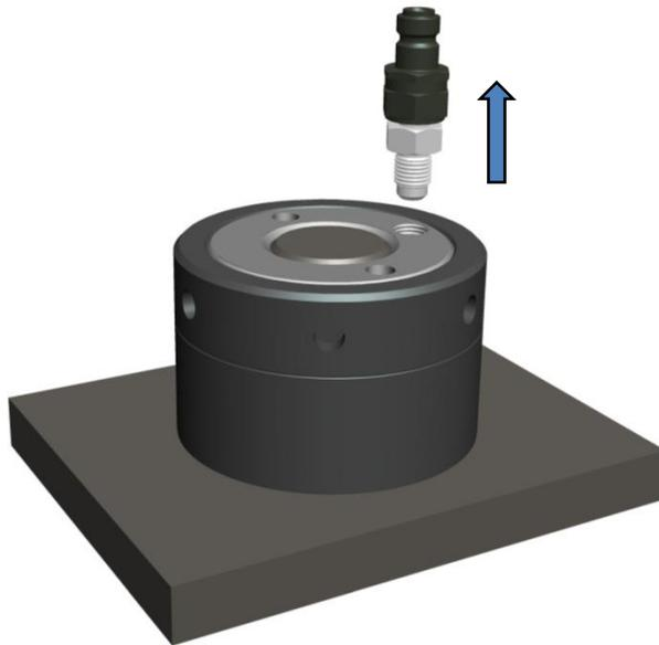
The Hydraulic Nut can be unscrewed.
