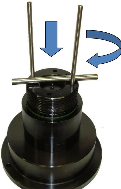
Use tommy bars to screw the Piston down into the Nut Body
