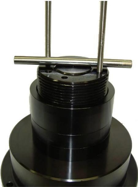
Screw the Piston fully into the Nut Body.
