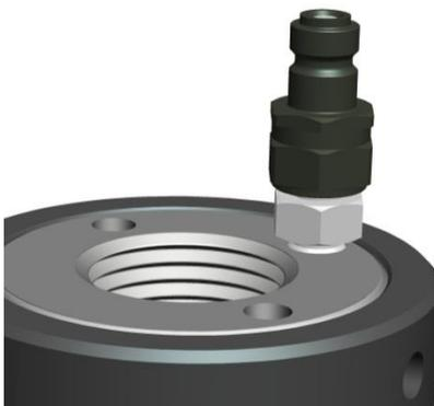
Using a spanner, firmly tighten then the nipple or coupling onto the adaptor. Take care not to over tighten the adaptor into the Nut.
